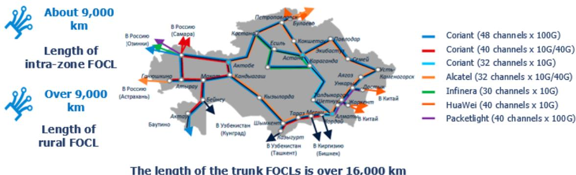
**Figure 1 - Transport network of Kazakhtelecom JSC (July 2020)**
